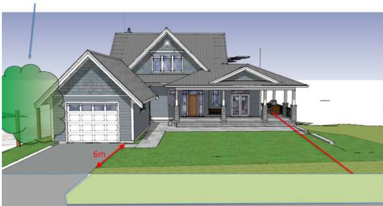
Figure 4: Building Drawings (red line shows required side yard setback from Eel Road)
